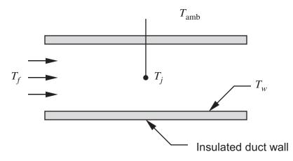
The junction exchanges heat with its surroundings by conduction, convection and radiation. Is  $T_j = T_f$ ?
