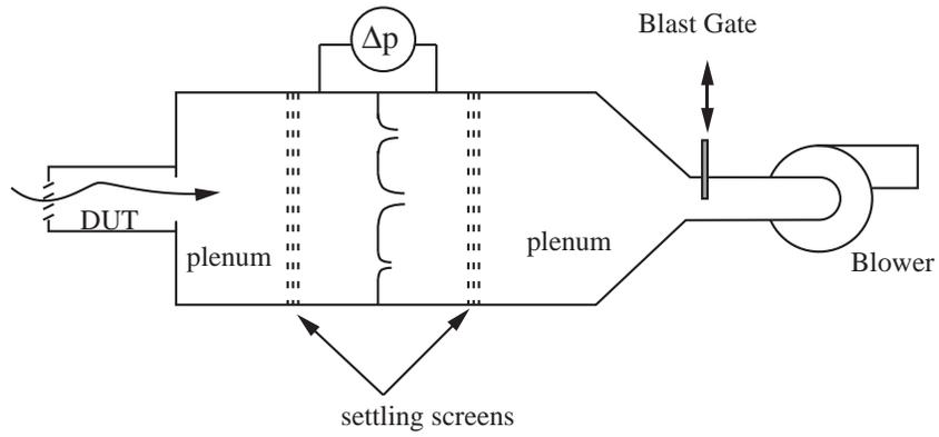
Figure 1: Flow bench schematic
