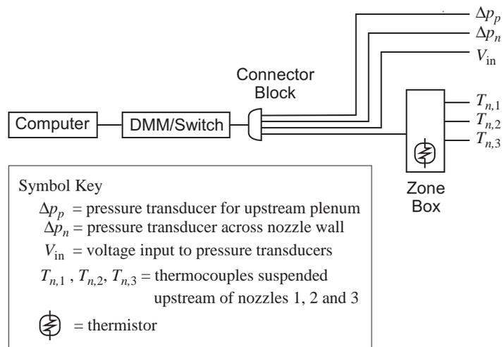
Figure 2: Block diagram for flow bench instrumentation
