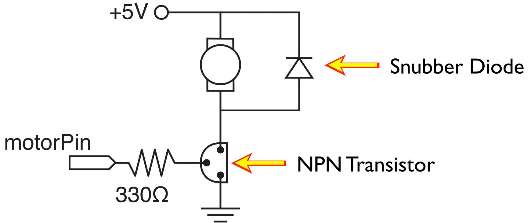
Add this to the breadboard with the potentiometer circuit
